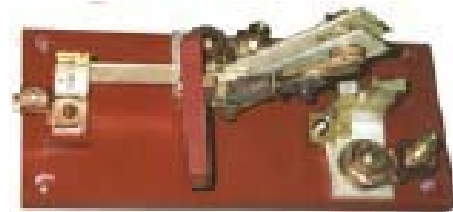
600 AMP 1000 VDC DISCONNECT WITH AUXILIARY BLADE TO GROUND LOAD TERMINAL IN THE OPEN POSITION FOR ENCLOSED EXTERNAL HANDLE OR HOOKSTICK OPERATION
